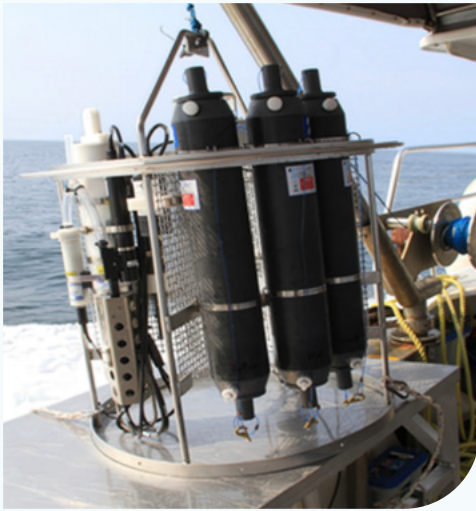
(a) CTD profiling instrument, dissolved oxygen sensor (attached to left side of steel frame) and Niskin rosette used to collect water samples (attached to right side of steel frame)
