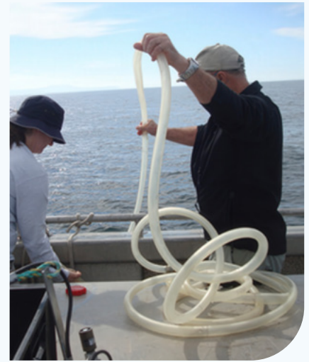
(c) Lund tube for collecting depth-integrated water samples from the surface
