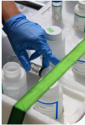
(b) preparation of syringe to filter particulates from raw water samples prior to analysis of soluble nutrients
