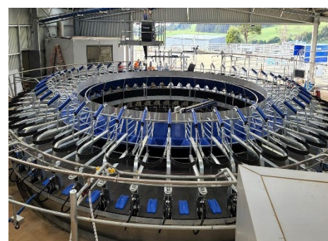
Image caption: TDRF operates with a 50-bail DeLaval rotary dairy.
