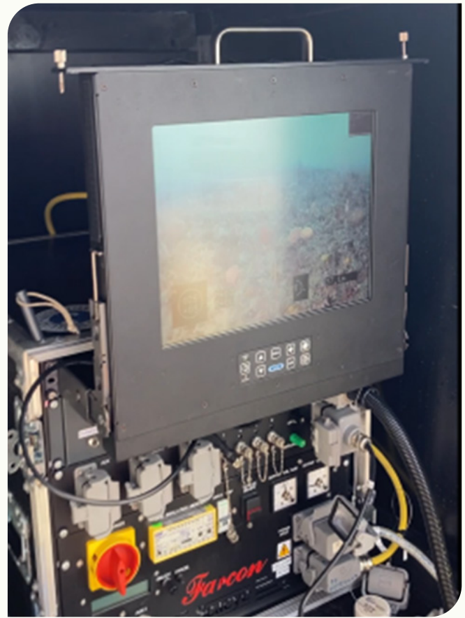
b) Falcon ROV control unit.
