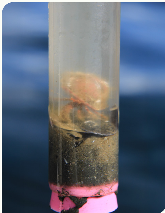
Figure 6: Perspex corer with an internal diameter of at least 50 mm
